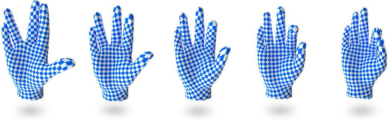
Fig. 1. Our formulation is combined with a projected Newton solver to interpolate from a Vulcan salute (left) to an OK gesture (right). We can also compute effects like surface parameterizations, elastic deformations and more using our algorithm. These are achieved by deriving an novel expression of the ARAP/corotational energy, which is written in terms of invariants of the Cauchy-Green tensor and thus free of numerically factored rotations and their gradients.
